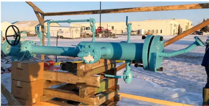
FIGURE 2: PIG LAUNCHER AND PACK-OFF HANGER ATTACHMENT
